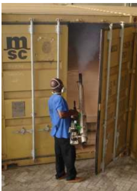
b. Space treatment with a pyrethroid UL formulation: using a thermal fogger before closing the container
